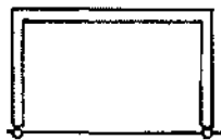
Rigid frame A structural frame of linear members rigidly connected at their joints. Applied loads produce axial, bending and shear forces in all members of the frame since the rigid joints restrain the ends of the members from rotating freely. In addition, vertical loads cause a rigid frame to develop horizontal thrusts at its base. A rigid frame is statically indeterminate and rigid only in its plane. Also called moment-resisting frame.
