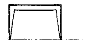
portal A rigid frame of two columns and a beam defining a single bay. Also called single-bay frame.
