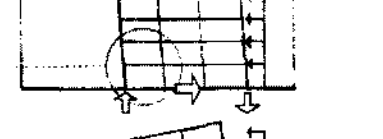
transfer column A vertical series of superimposed rigid frames, supported at some intermediate level where its load is transferred to adjacent columns.
